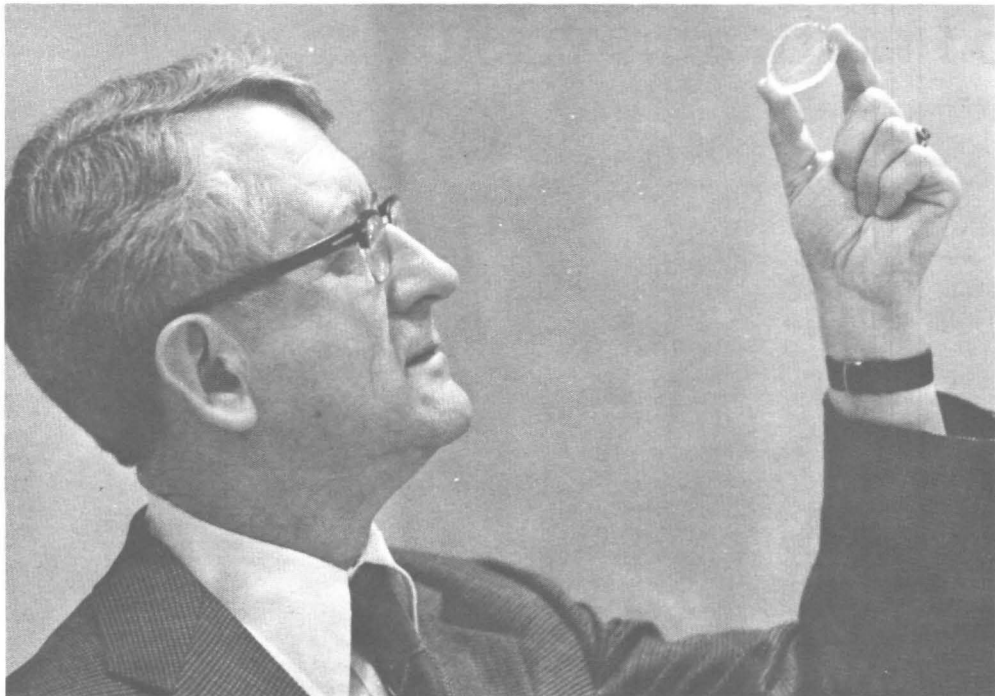
Dr. Frank Verbanac holds lens-like material prepared in seconds by passing ultraviolet light over the "Starpol" 100 solution.
