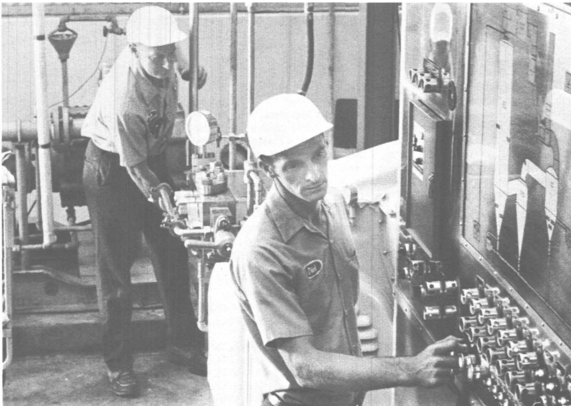
New flash dryers finish the soy albumen to a flour-like material—the state in which it will be shipped to customers for use as a whipping agent. Maintenance superintendent Dick Fennig, left, checks a pump on the system and Dick Gorham, a foreman, looks over the dryer panel board.
