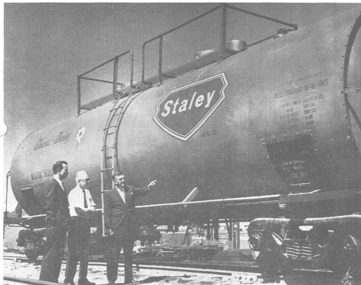
DAISY'S DEBUT —World's first all stainless steel syrup tank car readies for initial loading at Staley plant. Discussing car's features are, from left, Director of Distribution Bob Schuermen , Clark Gidel , Chief Shipping Inspector, and Corn
