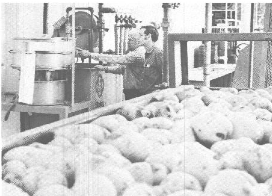
Paul Neumann, left, and Steve Tyler check the operation of the new dry starch recovery unit at Perfect Potato Chips, Inc. Paul is plant manager at Monte Vista, which processes most of the starch recovered at Perfect and in similar operations. Steve is a chemical engineer and did much of the development work.
