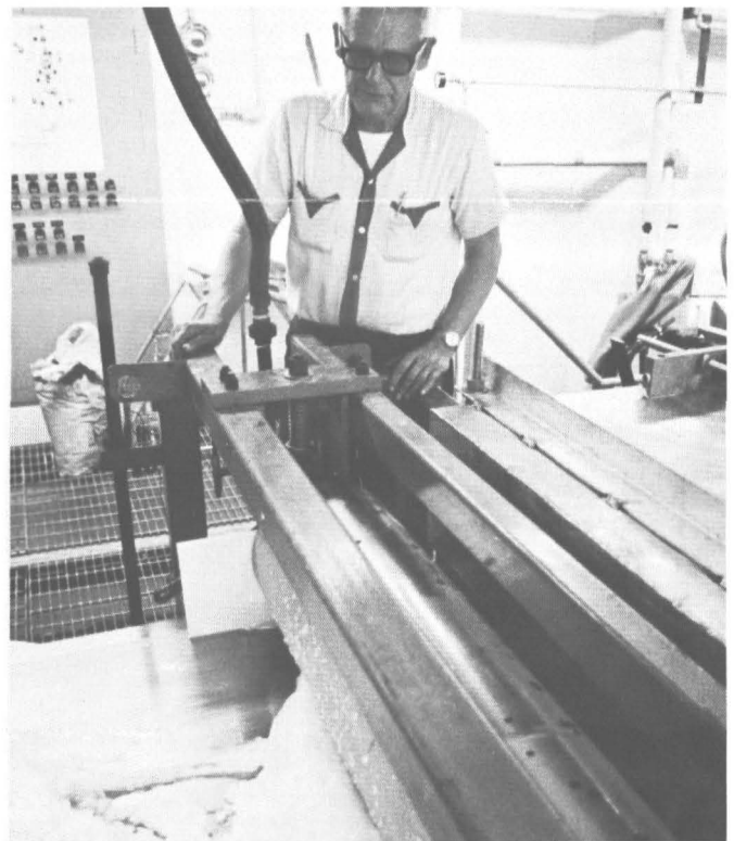
Molten corn syrup before it enters the evaporation system Operator Bernard Runyen checks for even distribution by the roller
