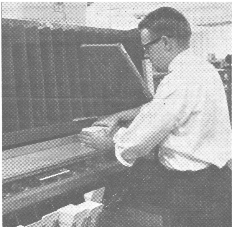
Doug Precht, unit record equipment operator, runs a batch of punchcards through sorting machine. Cards are coded for machine sorting. Cards are sorted by project for easy retrieval of information they contain.
