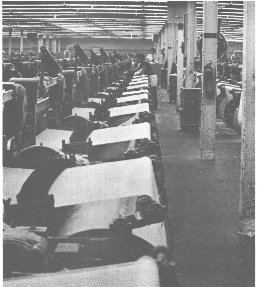
Some of the more than 1,200 looms in one giant room working almost non-stop at Clinton Mill's plant in Clinton, S. C. The repeated action of the shuttle against the thread is made possible by the strength imparted the material by Staley starch.
