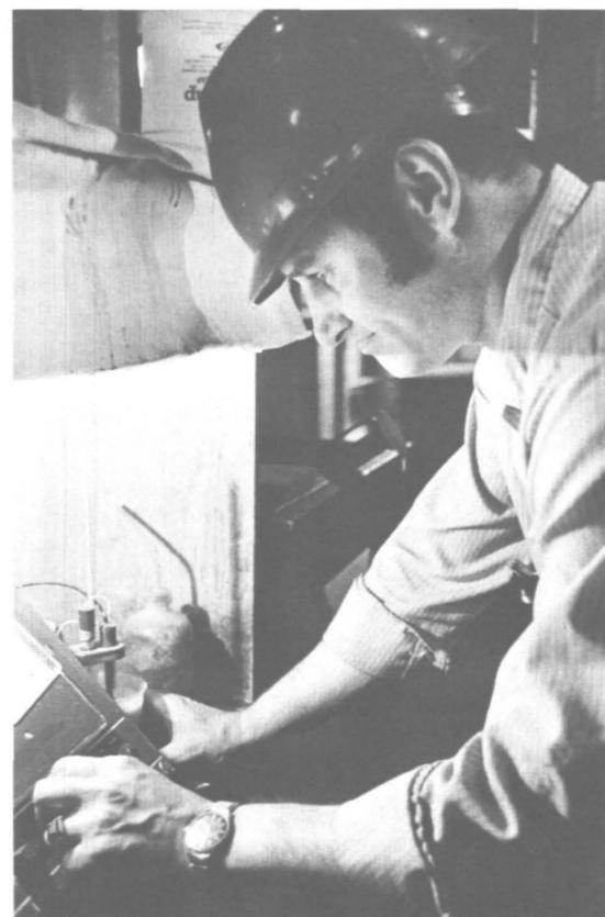
Operator Willard Goff reads a meter checking the acidity level during the making of Inositol.
