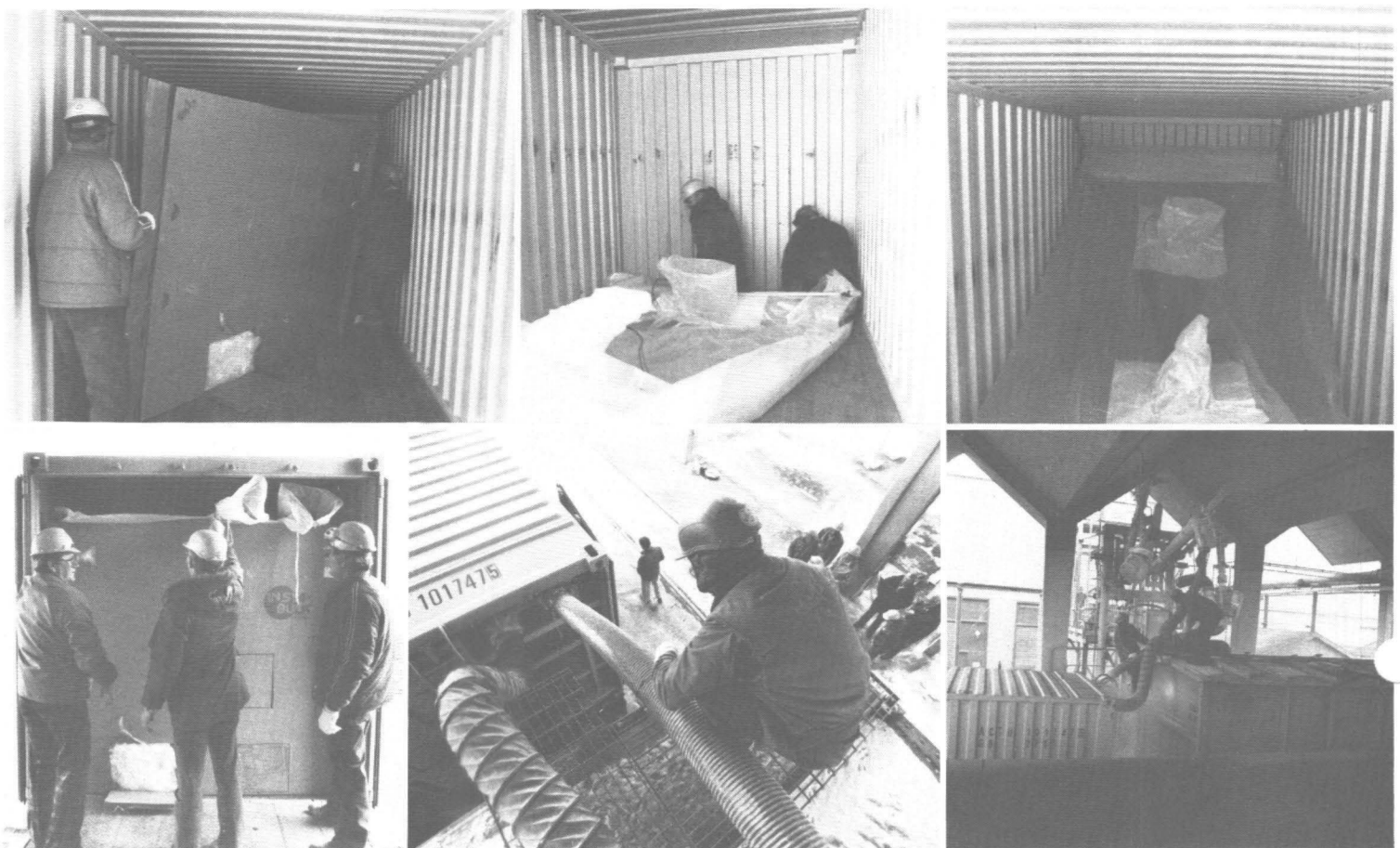
Sagamore employees are shown preparing and loading a 40,000-pound bulk container of starch for export to Australia. To give the product an air-tight ride, they installed a 20-foot-long plastic bag, into which the starch was loaded.
