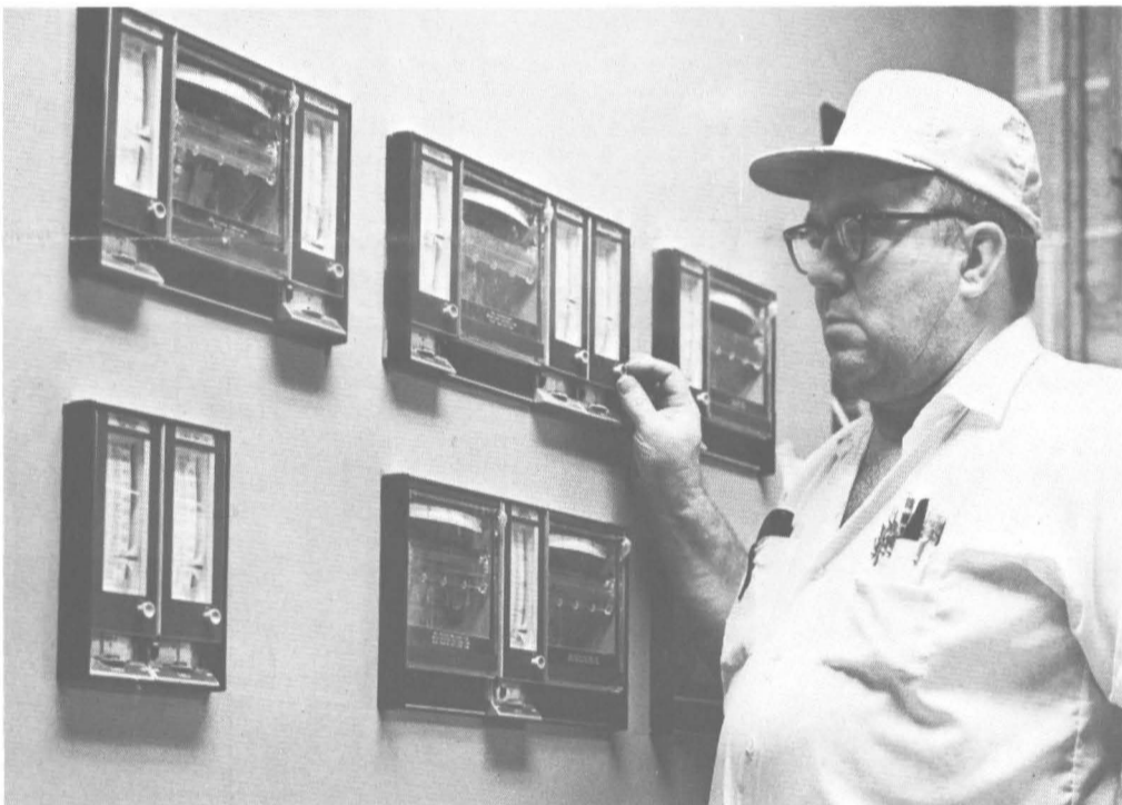
Charles Phegley Monitors the Flow at Control Panel Incoming Starch and Chemicals are Metered Automatically
