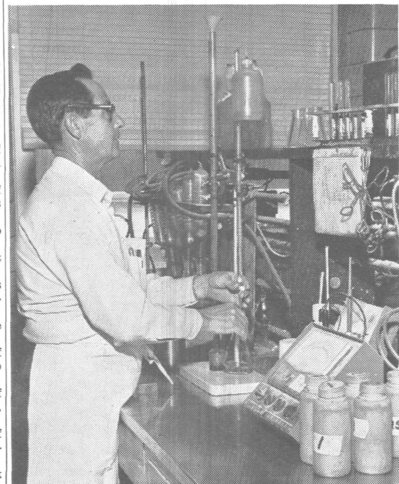
CONTROL LAB TESTS —Maurice Smith adjusts laboratory apparatus in preparation for testing waste flow samples as part of the Company's sewer loss reduction program. Reductions in plant sewer losses have been dramatic during the past year. (Related story and photos on Page 5.)
