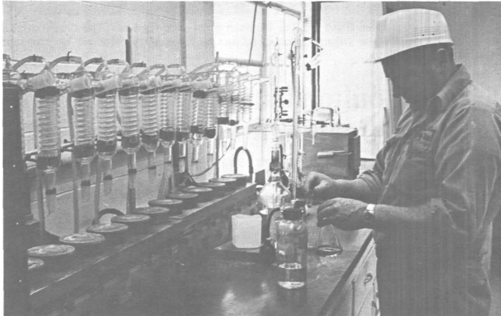
Checks of waste water standards are made on both a cumulative and spot basis in the plant's laboratory.
