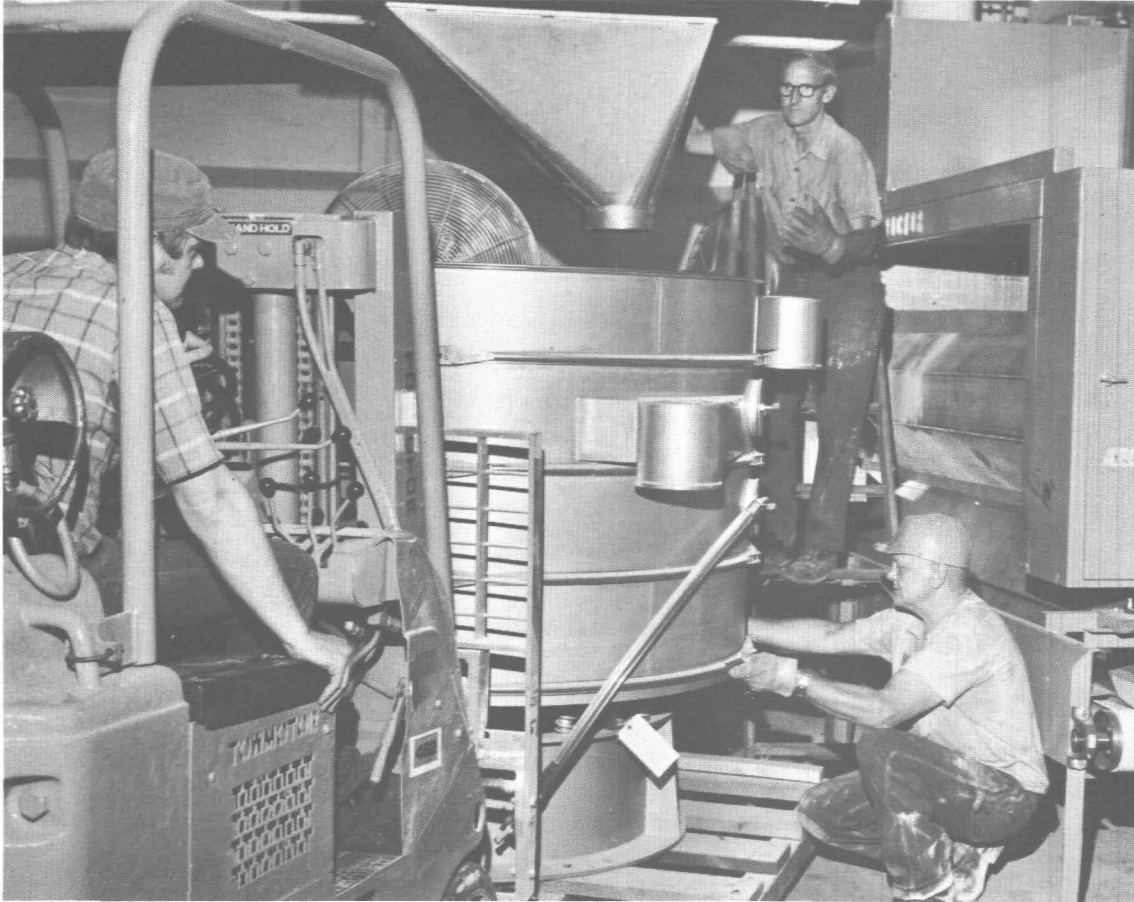
Completing installation of the sifter which grades the finished textured protein according to size are, left to right, bag dumper cleaner J.B. Webb, Bob Craig and M.W. Williams, both rigger leadmen. The sifter is part of the new process installed in 48 building.
