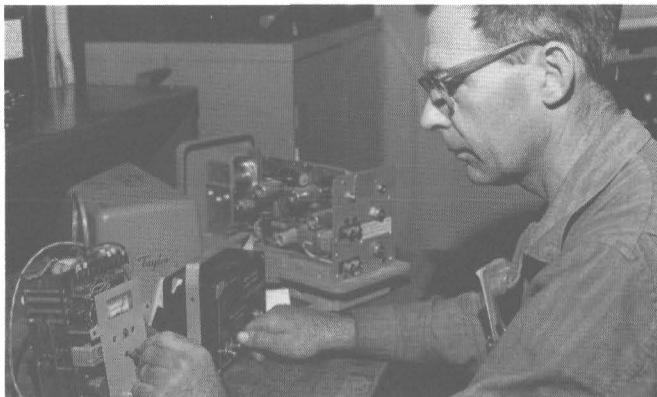
Donald White Calibrates a Magnetic Flow Meter
