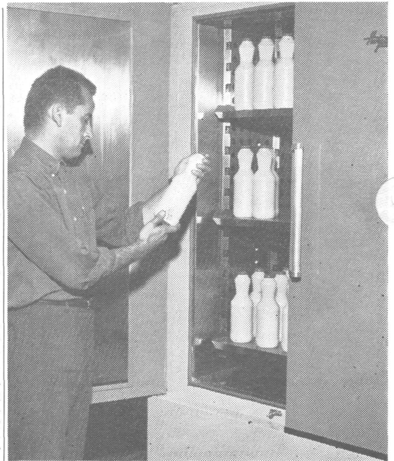
STRESS TEST —Les Carr, industrial engineer, looks at "Sta-Puf" plastic bottle to see how well it is resisting stress cracking under high heat conditions. This test is conducted on our plastic bottle supplies to assure they are capable of withstanding heat in transit and storage without cracking and leaking.
