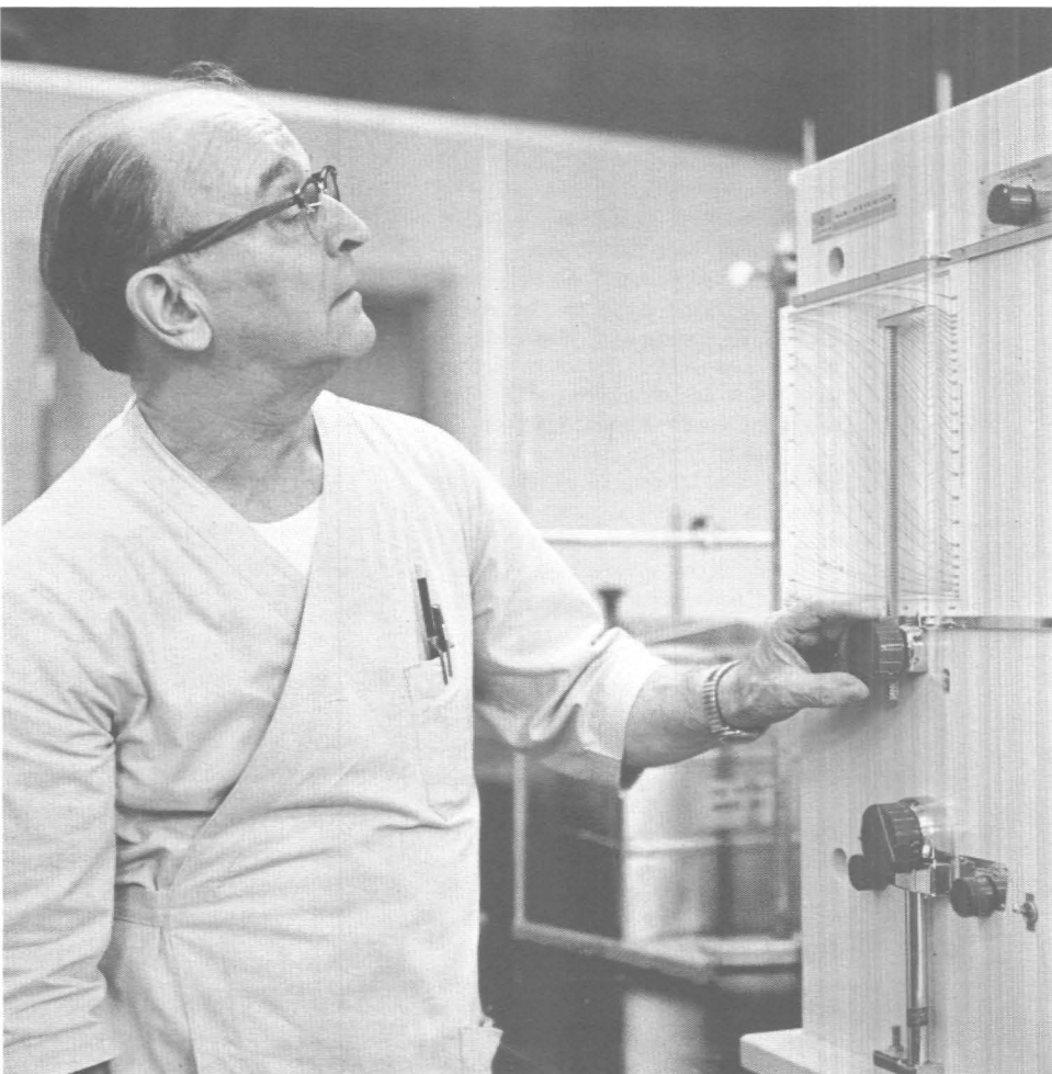
Jim Todd checks particle size of wheat granules. The testing device is accurate to 1/25,400 of an inch.
